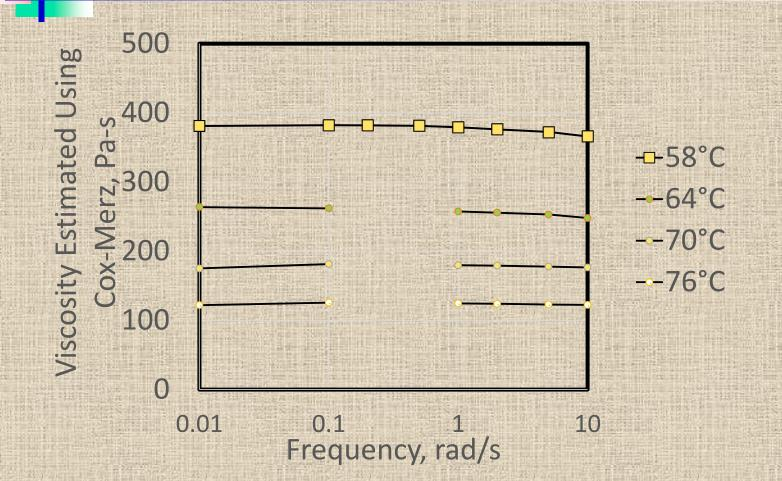
Shear thinning starting at 64°C increasing at 58°C
