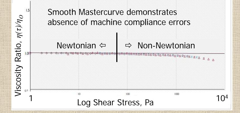
Non-Newtonian apparent when shear stress > 100 Pa
